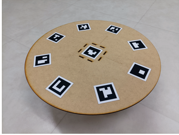
Figure 7: Calibration board for the transformer node.
