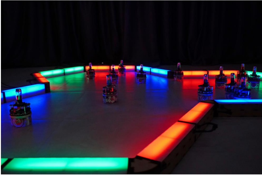
Figure 1: MoCA: a modular RGB color arena for swarm robotics experiments.
