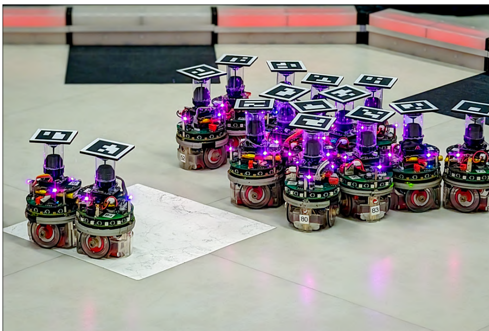
Figure 2.1: Swarm of e-puck robots. All studies presented in this dissertation are based on the e-puck.
