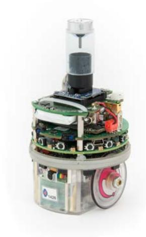
Figure A.1: **E-puck extended with range and bearing, Linux extension board and omni-directional camera.**
