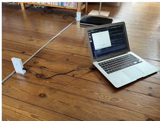
Figure 5.3: Experimental setup for analyzing the static distribution of the RToF estimated distances.
