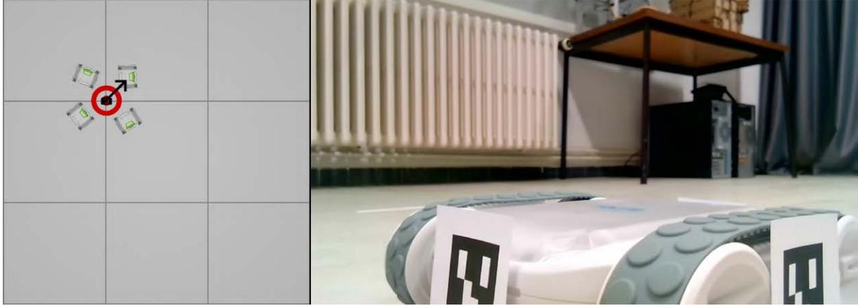
Figure 6.17: *ArUco* markers not fully visible on a close robot
