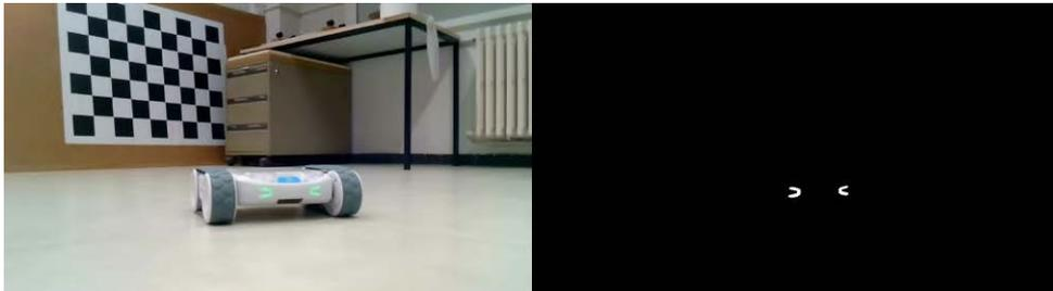
Figure 5.2: Colour segmentation using the LEDs of the *Sphero RVR* robot
