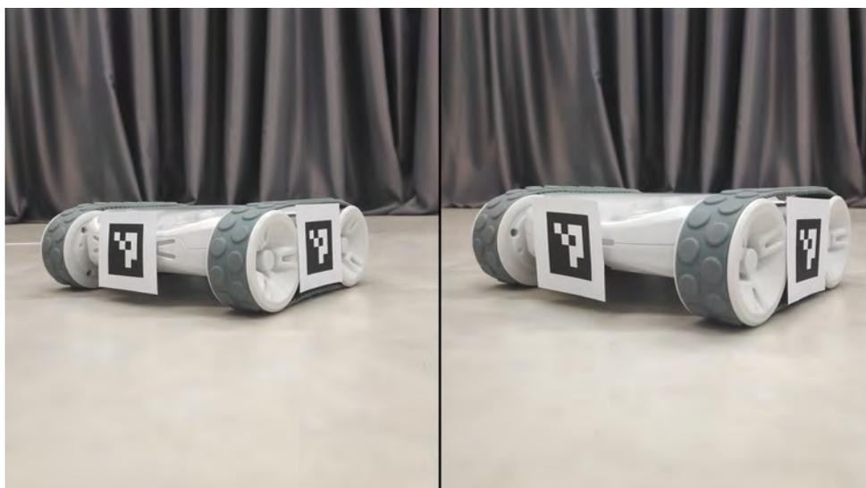
Figure 5.4: Placement of the *ArUco* markers on the *Sphero RVR* robot
