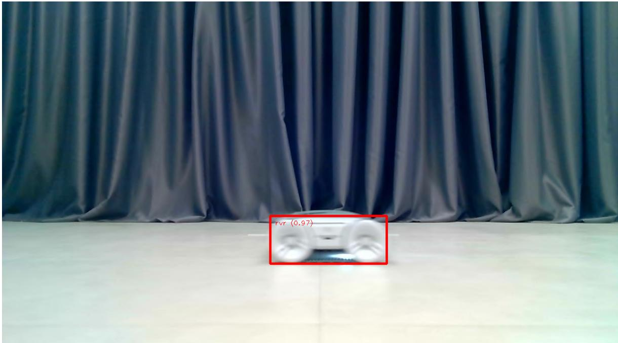
Figure 7.4: *Sphero RVR* robot with motion blur detected by the neural network
