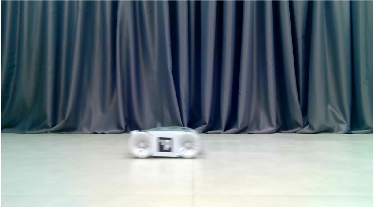
Figure 7.3: Motion blur on a *Sphero RVR* robot with *ArUco* markers
