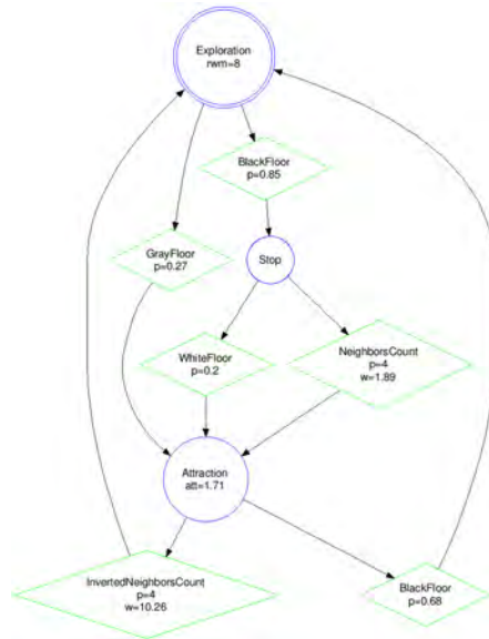
Figure 3.1: Finite state machine generated by AutoMoDe for an aggregation mission. The robot controlled by this finite state machine explores the environment and stops when it finds a black spot. It also tends to be attracted to its neighbors when it counts multiple surrounding robots.
